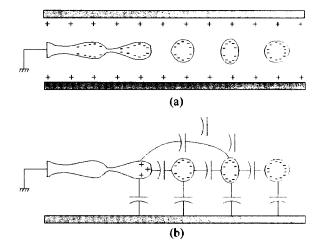
Figure 3. Charging geometry for a typical CIJ system.
