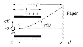
Figure 4. Representation of a deflection system.
